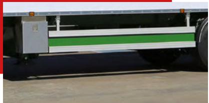
Painted metal plate between cyclist guards
