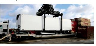
Combined road-rail transport: system for loading a complete semi-trailer on a pocket wagon
