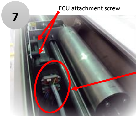
Attachment of electronic module and connectors
